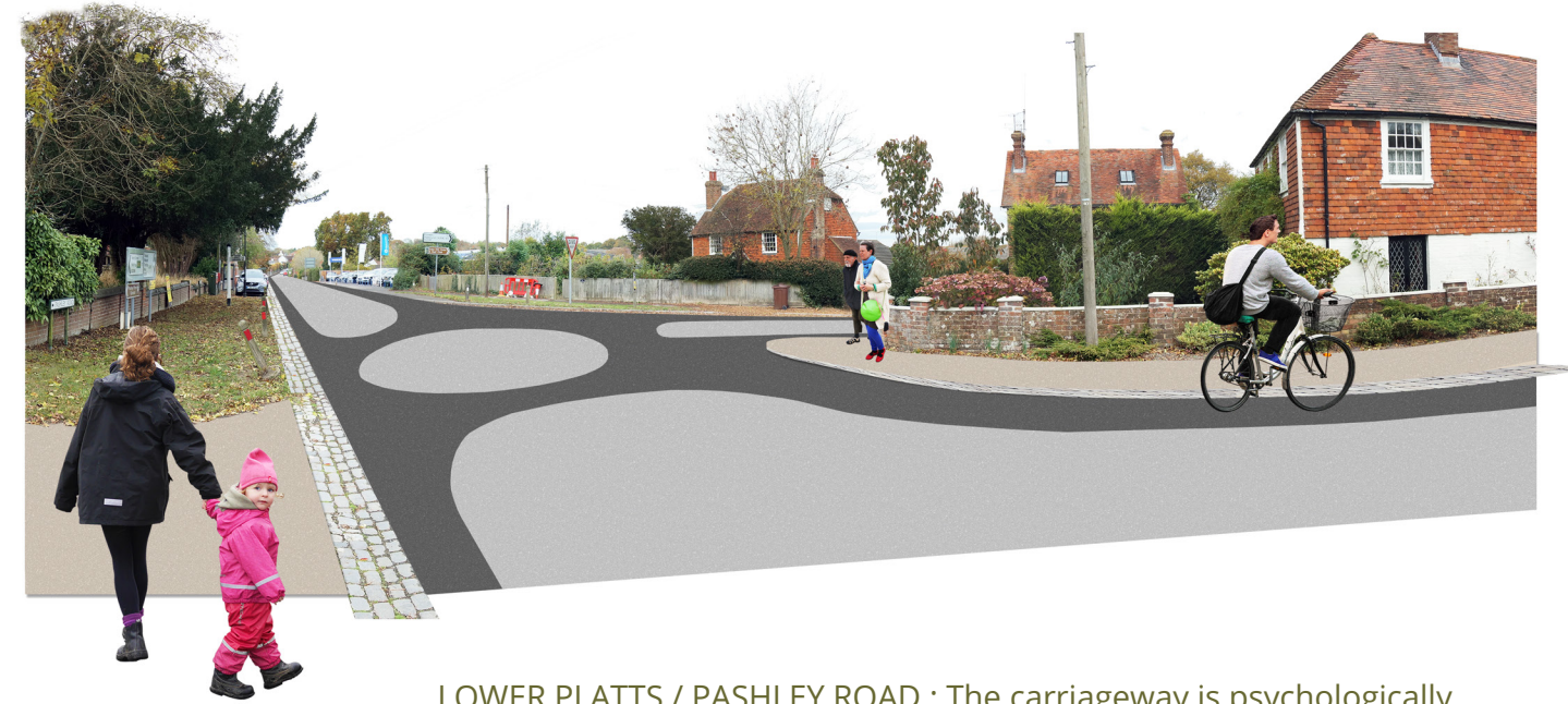
LOWER PLATTS / PASHLEY ROAD : The carriageway is psychologically narrowed by the new colours, causing drivers to slow down as they approach the junction. By alternating between differently coloured surfaces, the long straight visual path is disrupted, removing the current temptation maintain a high speed through the village.
